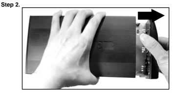
Carefully slide the Inner Cradle with PCB and Front Cover off the Body Outer Cover with Rear Panel.
